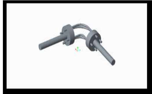
Fig 3.1 3D module of gearless transmission
